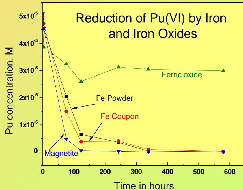
The presence of  $Fe^0$  and  $Fe^{2+}$  resulted in the rapid loss of plutonium from solution. In the case of ferric oxide some loss of Pu was noted, but residual concentrations remained high and it was (postulated) due to sorption not reduction/precipitation. The most complete and rapid loss of Pu occurred for magnetite which was the only iron phase that contained  $Fe^{2+}$ . These results show that  $Fe^0$  and  $Fe^{2+}$  effectively remove dissolved plutonium from brine.
