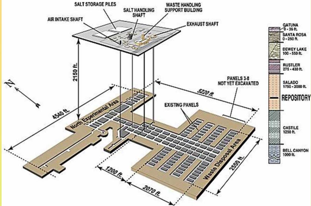
Disposal rooms are excavated in an ancient, stable salt formation 2,150 feet (almost one-half mile) underground. Transuranic waste, which consists of clothing, tools, rags, debris and other disposable items contaminated with radioactive elements, mostly plutonium, are emplaced in 55 gallon steel drums for permanent disposal.
