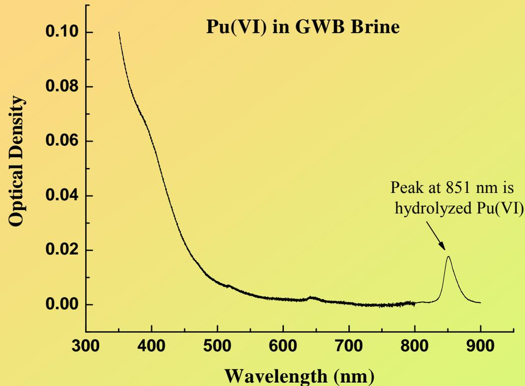
The absorption spectrum of the plutonium in GWB brine. Since the pH is ~ 9, the plutonium is hydrolyzed (complexed with hydroxide) resulting in a 20 nm shift in the absorption maximum to 851 nm. The absorption spectrum of this solution was stable over the three-month period that it was monitored.
